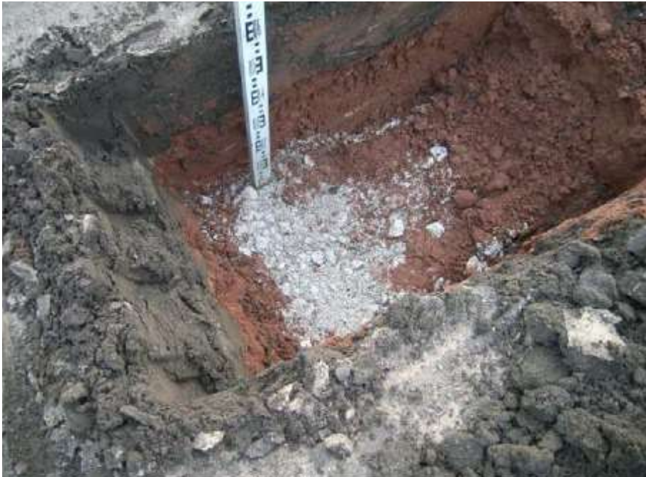
Photograph 8: Excavation within public open space and verification pit showing the presence of a remediation break layer at the base, a crushed sandstone inert fill overlain by topsoil.
