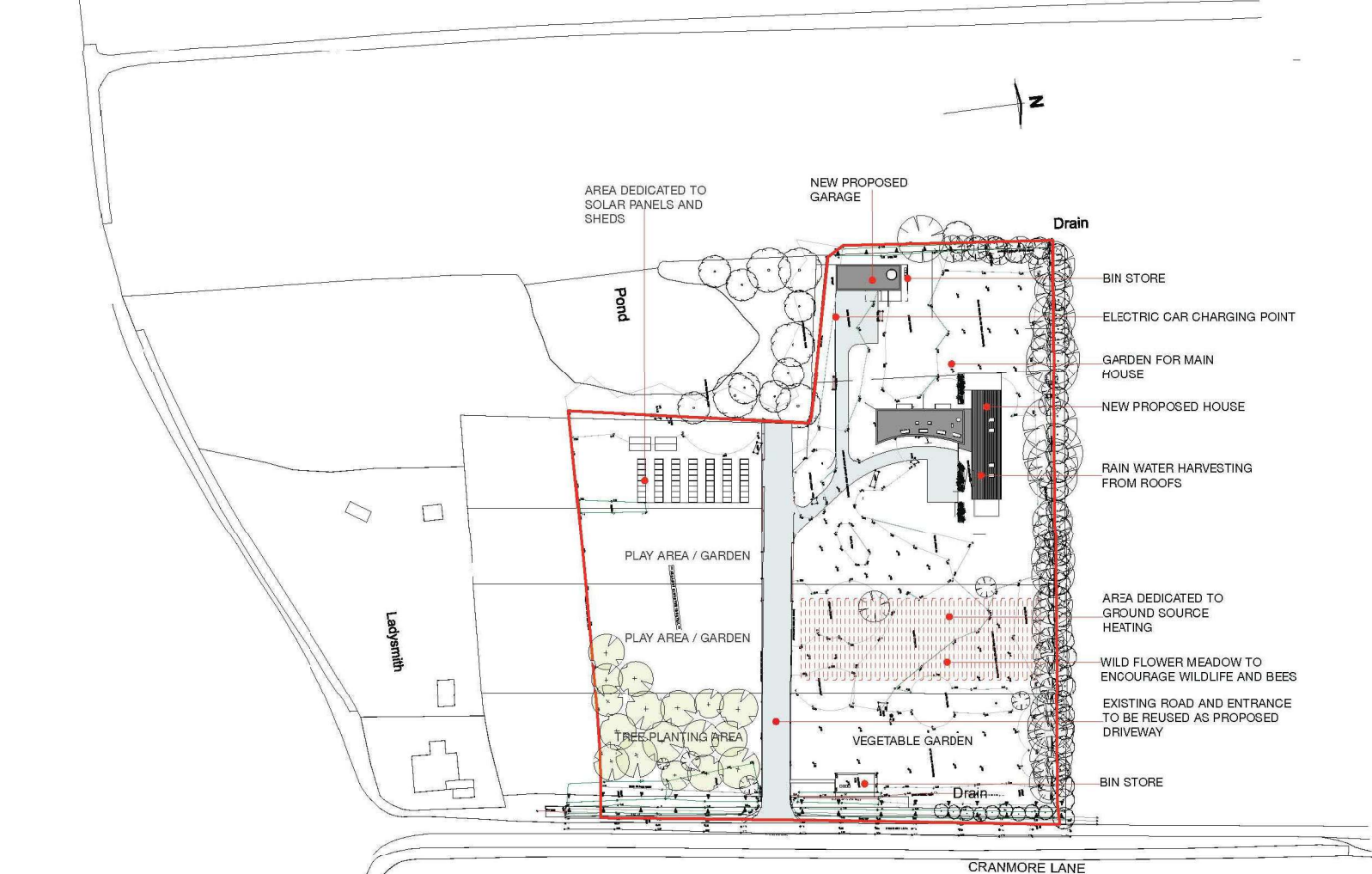
PROPOSED SITE & ROOF PLAN 1:1000
