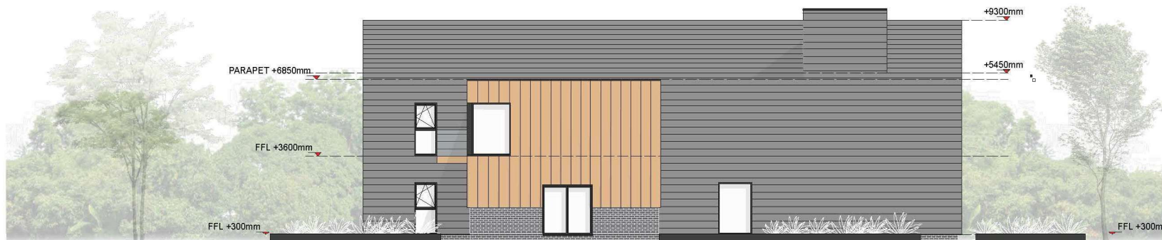
PROPOSED WEST ELEVATION 1:150
