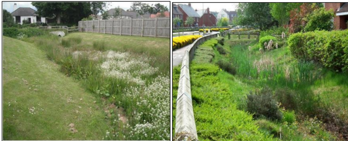
Figure 4-2: Examples of swales for drainage and biodiversity
